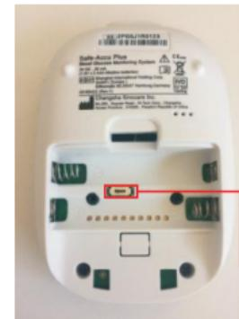
The Safe AQ Voice is preset as voice on. Slide the battery cover out of the meter. Remove the batteries. Voice switch is inside the battery chamber. Slide the voice switch to the "on" side, voice turns on and screen will display "♪" symbol when meter is on; while slide to the "off" side, voice turns off and screen won't display "♪" symbol.
