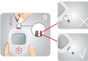
For Safe AQ Smart, Safe AQ Air, if the meter display “E-2”; for Safe AQ Voice, if the meter display “E-2” and play “The temperature is beyond the range”, it means the environment temperature is beyond the range. Please put the meter, strip, control solution at appropriate place (10°C~35°C), wait at least 30 minutes and test again.
